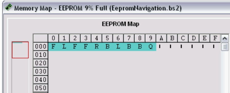
Figure 4-8 Close-up of the Detailed EEPROM Map after Display ASCII Box is Checked
